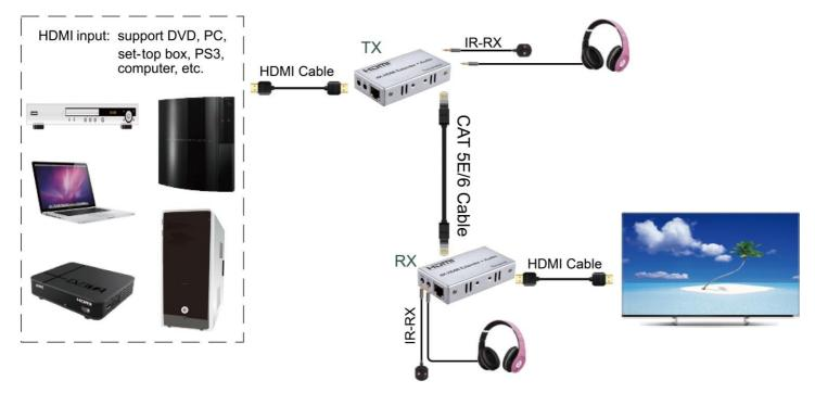
Connect one HDMI cable between your source device and the TX Extender (Sender), the max cable length is 15 meters.
